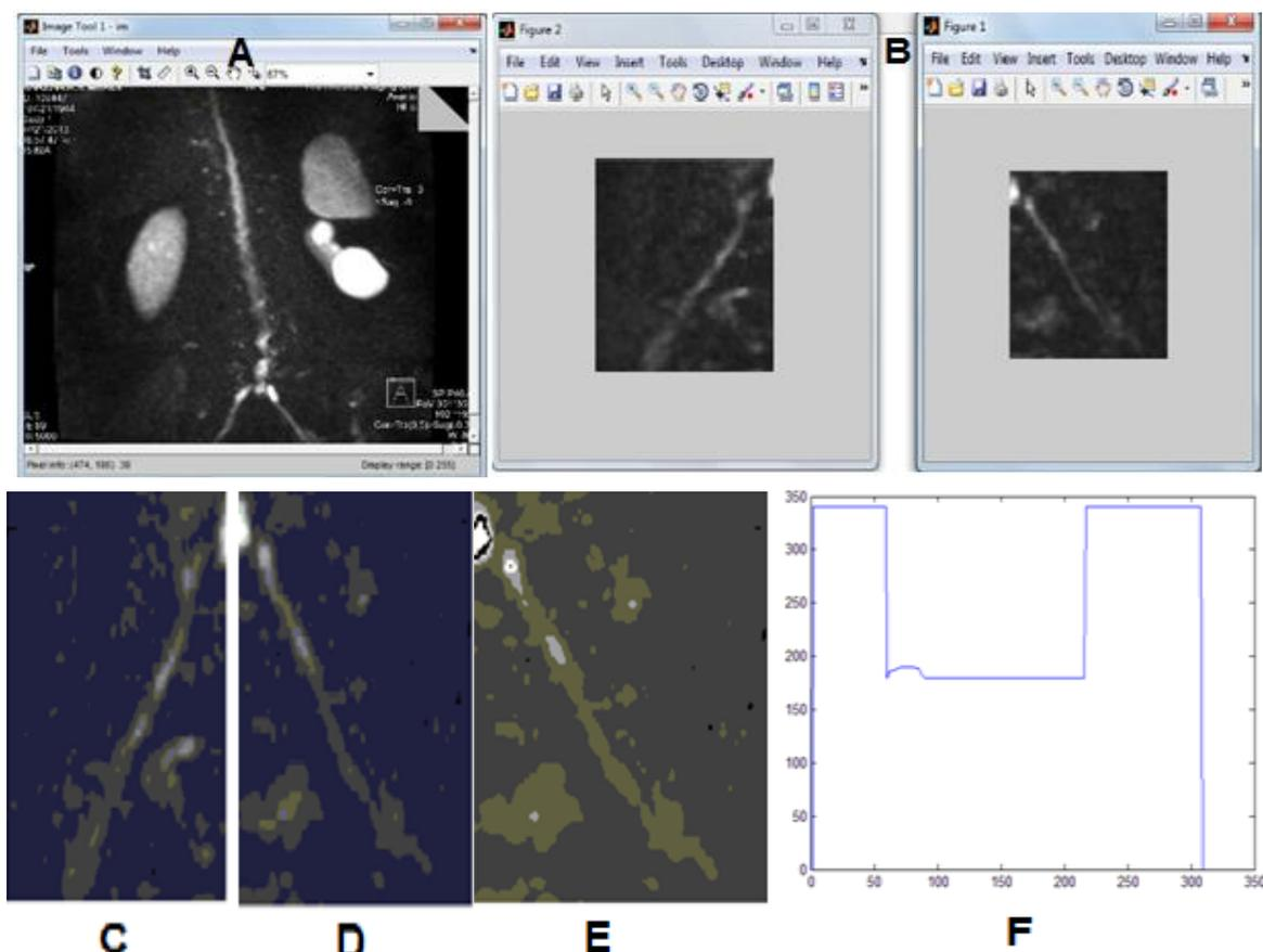
**Figure 3.** Different levels of image processing in MATLAB software. A) Illustrates the image selection and finding a start point. B) Illustrates the image division. C, D) Noise elimination and smoothing. E) Otsu matrix module and Binary conversion. F) The chart of changing nerve diameter on one side in selected length.
