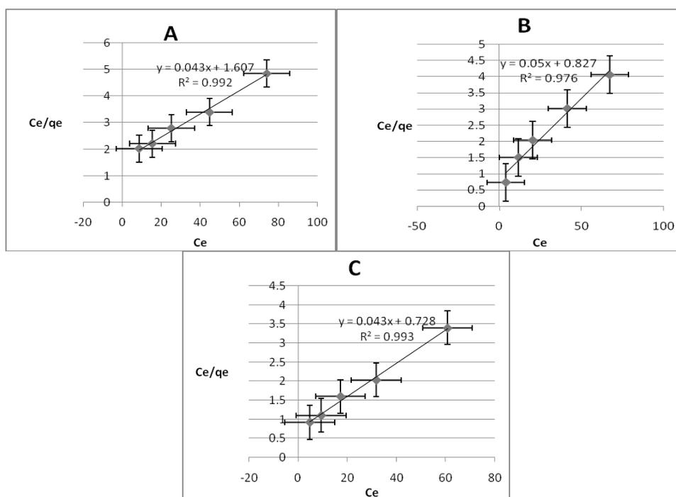
**Figure 2.** Langmuir adsorption isotherm for Cd (II) ion biosorption onto (A): *L. muralis*, (B): *A. strigata* and (C): *C. aurantia* [( $C_e/q_e = 1/Q_{ob} + C_e/Q_b$ ),  $C_e$ : equilibrium concentration,  $q_e$ : amount adsorbed of Cd (II) at equilibrium,  $Q_o$ : Langmuir constants related to adsorption capacity,  $Q_b$ : Langmuir constants related to energy of adsorption].
