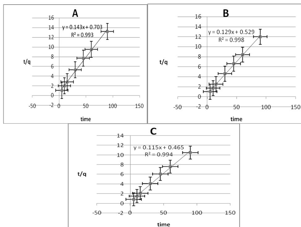
**Figure 4.** Pseudo-second-order kinetic plot for the biosorption of Cd (II) ions onto (A): *L. muralis*, (B): *A. strigata* and (C): *C. aurantia* [ $t/q = 1/Kq_e^2 + 1/q_e * t$ , t: contact time (min), q<sub>e</sub> (mg/g) and q<sub>e</sub><sup>2</sup> (mg/g): amount of solute adsorbed at equilibrium, K: the rate constant].
