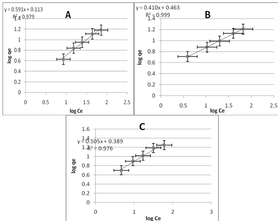
**Figure 3.** Freundlich adsorption isotherm for Cd (II) ion biosorption onto (A): *L. muralis*, (B): *A. strigata* and (C): *C. aurantia* [( $\log q_e = \log kf + 1/n \log C_e$ ),  $kf$ : constant relating the biosorption capacity,  $1/n$ : empirical parameter relating the biosorption intensity,  $C_e$ : final concentration at the equilibrium (mg/L),  $q_e$ : metal uptake at the equilibrium (mg/g)].
