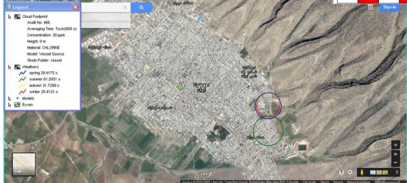
Figure 2. Maximum concentration footprint of chlorine on the Eyvan map for rupture of vessel.
