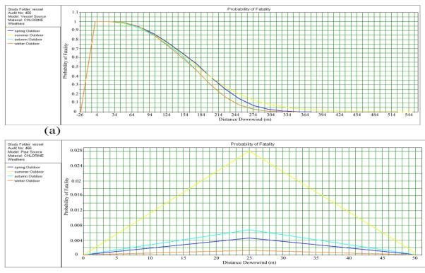
Figure 3. Probability of fatality for rupture of: (a) chlorine vessel (b) chlorine pipeline in four seasons.
