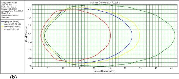
Figure 1. Maximum concentration footprint for rupture of: (a) chlorine vessel (b) chlorine pipeline in four seasons.
