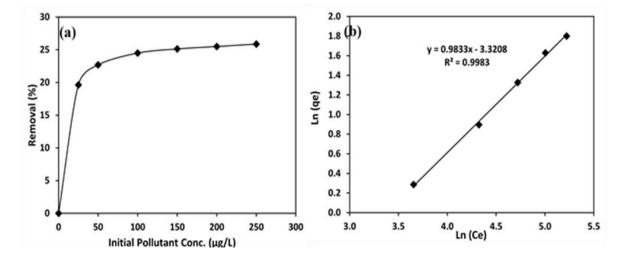
**Figure 3. (a)** The effects of lindane concentration on the adsorption by mineral sand (pH =4.0, contact time =150 min, solution volume =250 mL and adsorbent conc. = 2.5 g) and (b) Freundlich isotherm model.
