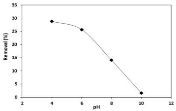
Figure 2. The effect of solution pH on the adsorption of lindane by the sand (lindane solution =  $100 \mu g/L$ , contact time =  $150 \mu g/L$
