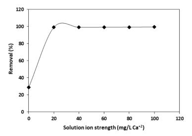
**Figure 4.** The effect of solution ion strength on the adsorption of lindane by the sand (lindane solution =  $100 \mu g/L$ , contact time =  $150 \mu g/L$ , solution volume =  $250 \mu g/L$  and adsorbent conc. =  $2.5 \mu g/L$  g).
